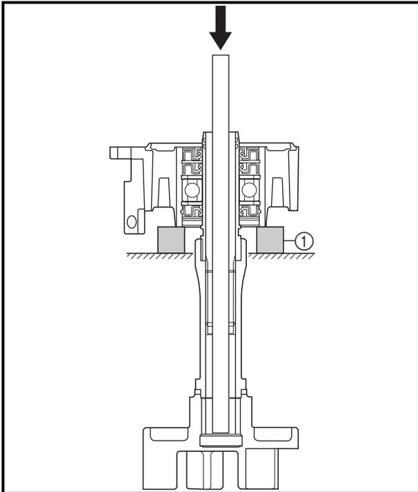
**Intermediate drive shaft removal**
