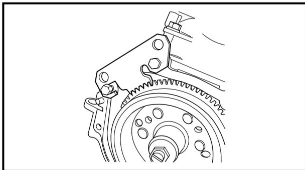
**Flywheel magneto removal and installation**
