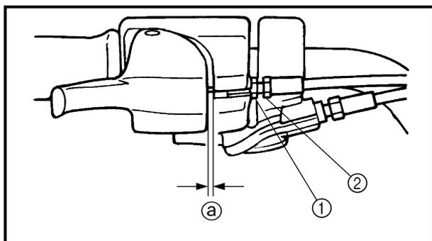
**Throttle cable inspection and adjustment**
