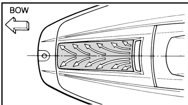
2. To prevent water from entering the urethane foam, apply silicone sealant to the inside of the hole as shown.
