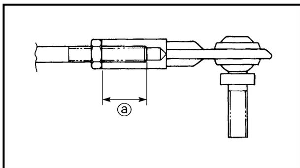
**Steering cable (jet pump side) installation**
