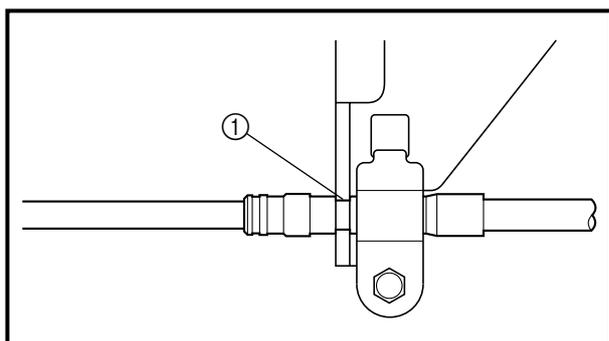
**Steering cable stopper installation**
