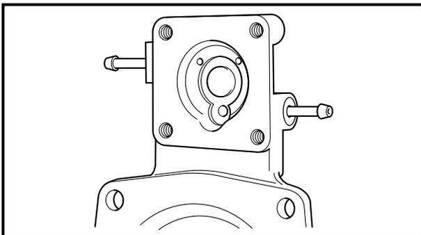
**Accelerator pump body inspection**
