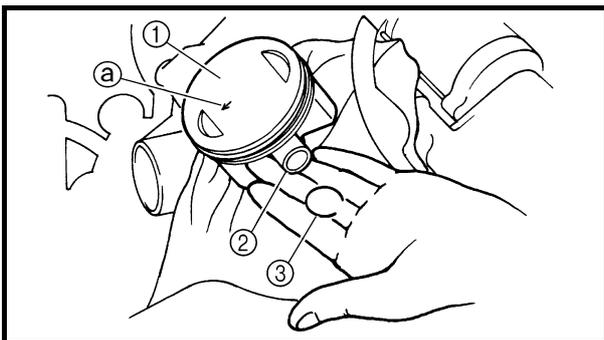
**INSTALLING THE PISTON**
