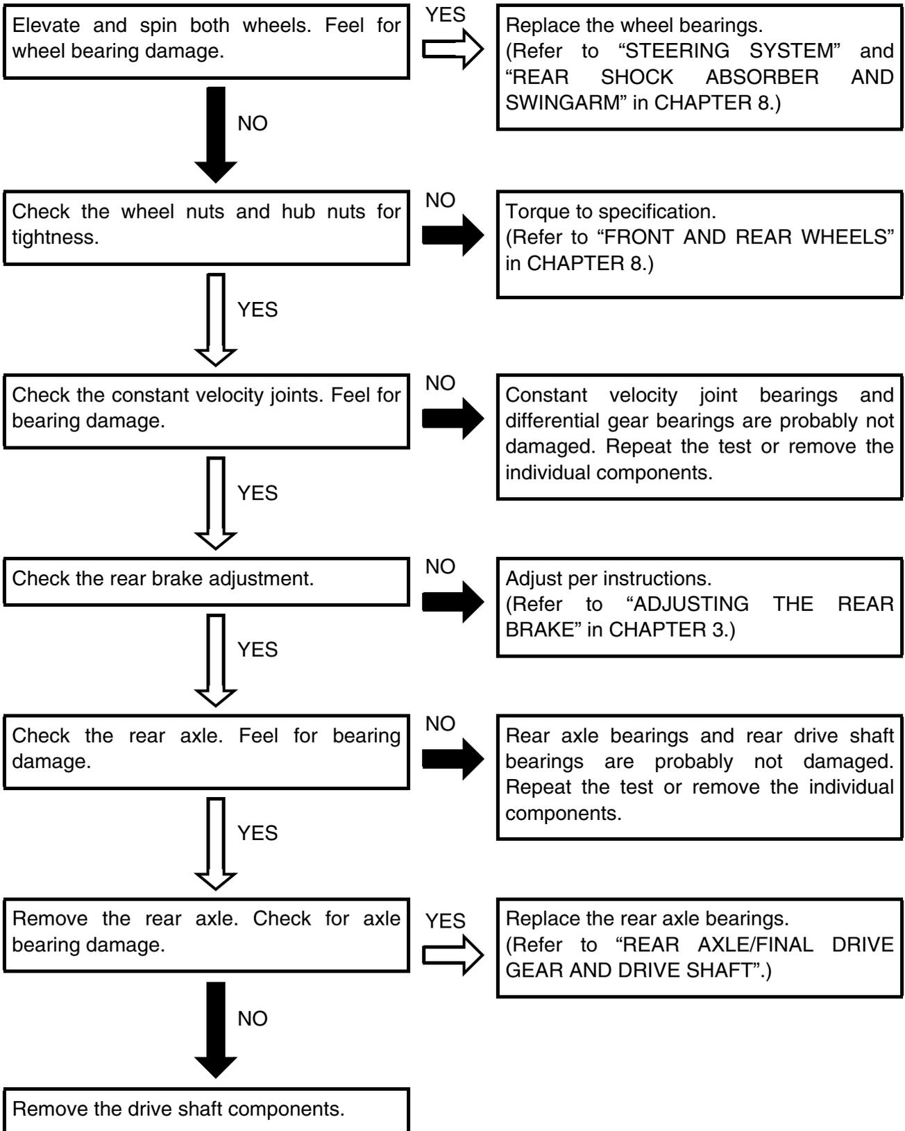
FRONT CONSTANT VELOCITY JOINTS AND DIFFERENTIAL GEAR
