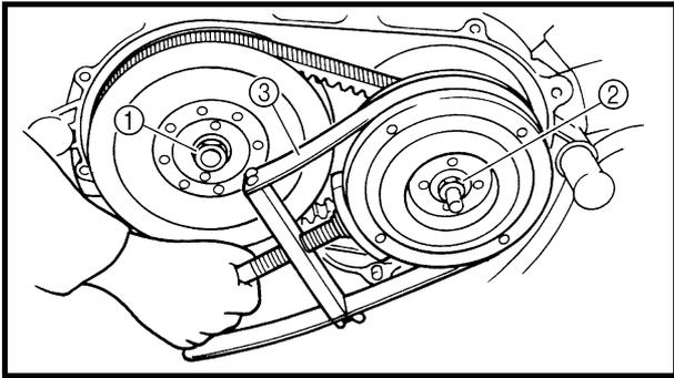
**REMOVING THE PRIMARY AND SECONDARY SHEAVES**
