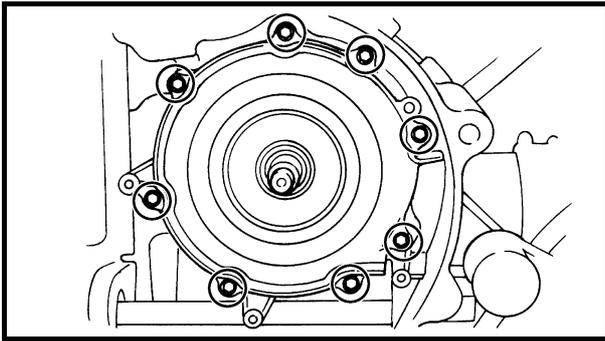
**REMOVING THE CLUTCH**
