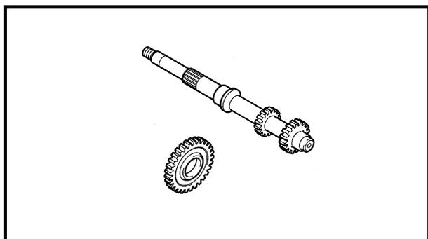
**CHECKING THE SECONDARY SHAFT AND DRIVEN SPROCKET**
