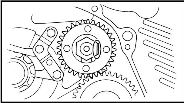
**REMOVING THE OIL PUMP DRIVE GEAR**
