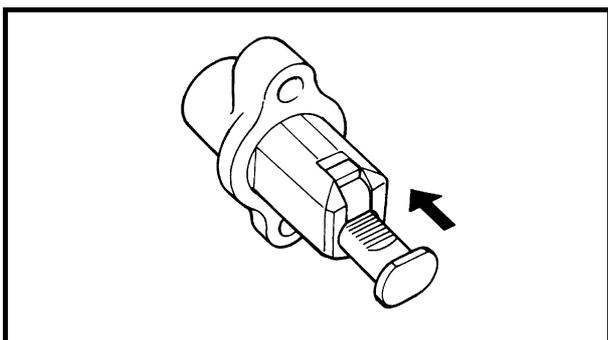
**CHECKING THE TIMING CHAIN TENSIONER**
