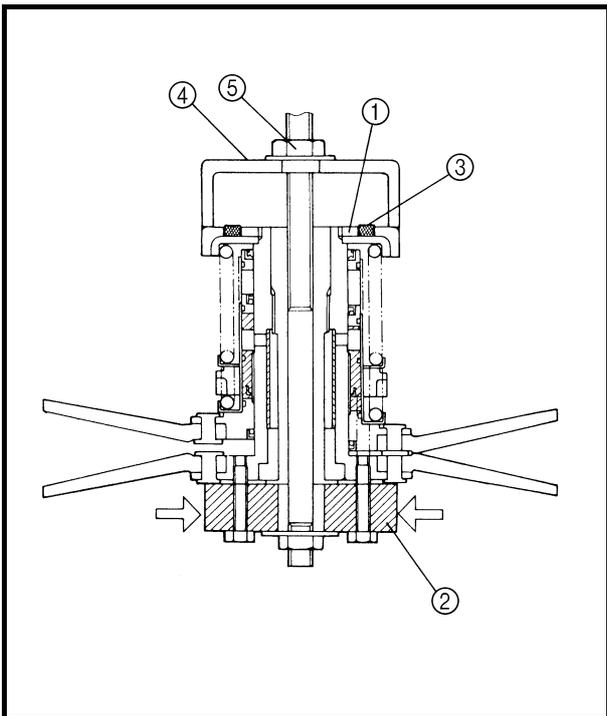
**DISASSEMBLING THE SECONDARY SHEAVE**
