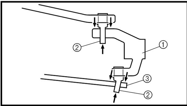
**REMOVING THE STEERING KNUCKLES**
