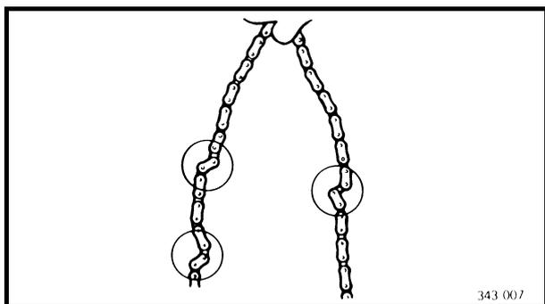
**CHECKING THE TIMING CHAIN AND GUIDE**
