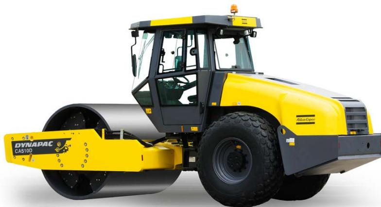
The Dynapac CA510 is a roller in the 18-ton class. CA510 is available in D (smooth drum) and PD (padfoot drum) versions. CA510D is intended for the compaction of rockfill. The main area of application for the CA510PD is on cohesive material and weathered stone material.
